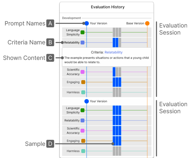
Figure 6: The history visualization is separated into sessions, which represent sets of samples that were generated and evaluated with the same prompts and criteria. For each session, the history shows the names of the prompts (A) and criteria (B) used, and the user can click on these to see their content at the time (C). For each criterion, the history shows a bar for each sample evaluated (D), which is color-coded to represent which prompt won or if there was a tie for that sample.
